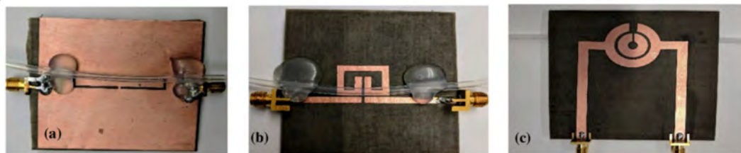
Figure 10. The geometries of the proposed three sensors, based on the complementary split ring resonator (CSRR) (a), extended gap SRR (EX-SRR) (b), and circular SRR (c) [98]. Reprinted from Sharafadinzadeh, N.; Abdolrazzagh, M.; Daneshmand, M. Investigation on planar microwave sensors with enhanced sensitivity from microfluidic integration. Sensors Actuators, A Phys. 2020 , 301 , 111752, doi:10.1016/j.sna.2019.111752 with permission from Elsevier.
